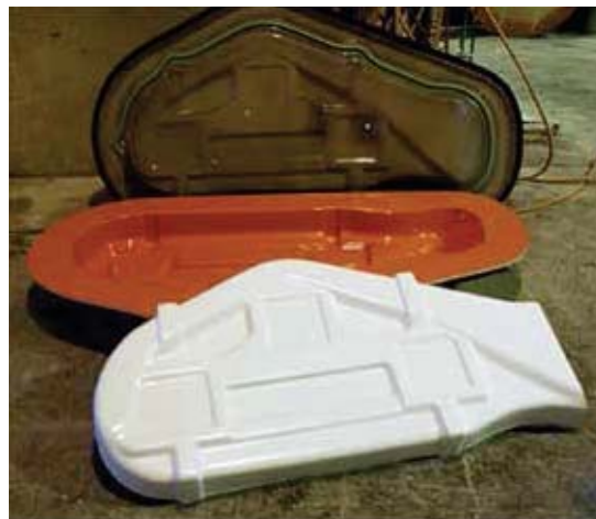
Figure 1 – Foreground - Finished Part; Middle - Base or “A-side” Mold; Back - Counter mold or “B-side” Mold
